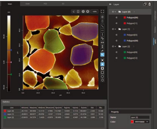
LTPS TFT backplane Topography Multiple Areas of Interest Assigned
